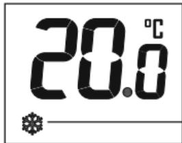
Frost symbol will continuously flash when frost mode is active
