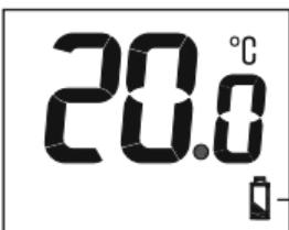
Battery low indicator will appear when the batteries are low.
