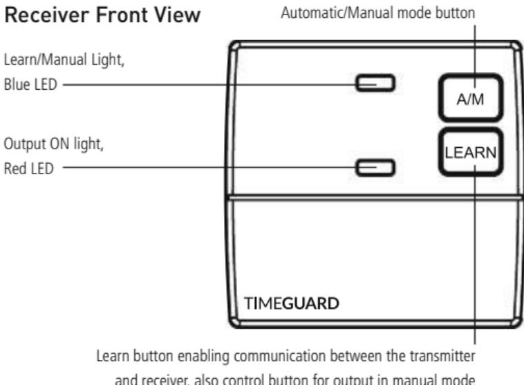
Learn button enabling communication between the transmitter and receiver, also control button for output in manual mode
